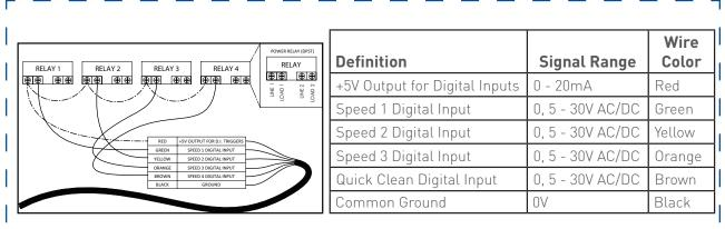
Figure 4. External Control Kit Wiring Diagram
